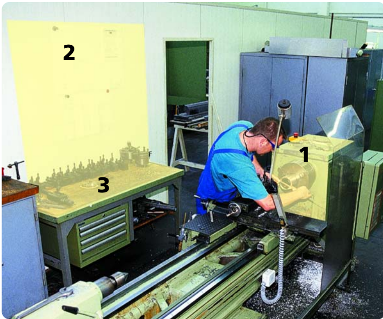
Fig. 9: Examples of task areas meeting different workplace requirements: space for turning and measuring moderately fine parts presenting vertical and horizontal visual tasks (1), place for studying drawings on vertical surfaces (2), place for checking workpiece measurements and depositing tools (3)
